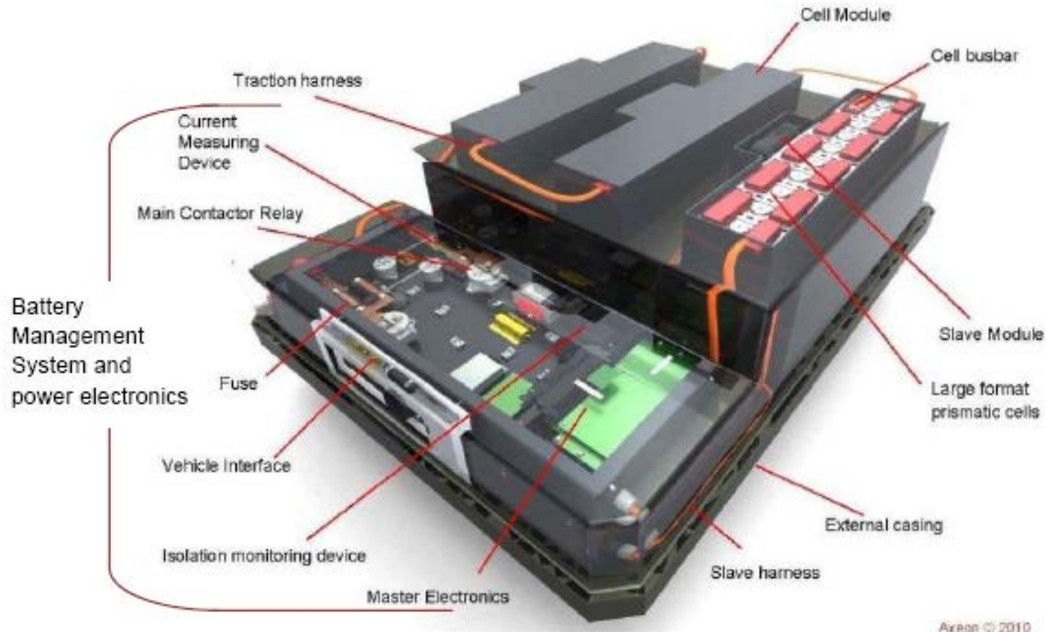
Figure 2-3 Example of a battery pack. Source: Axeon guide to batteries
