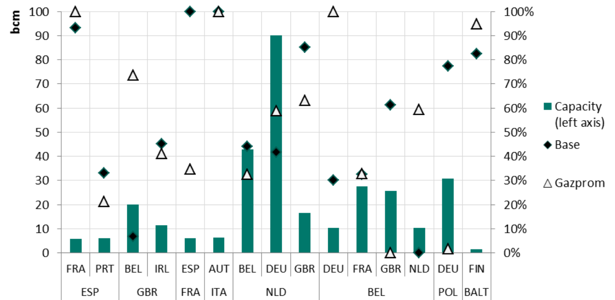
Figure 24: Pipeline capacities (left axis) and export utilization rates from LNG importing countries, in bcm and percentages.
