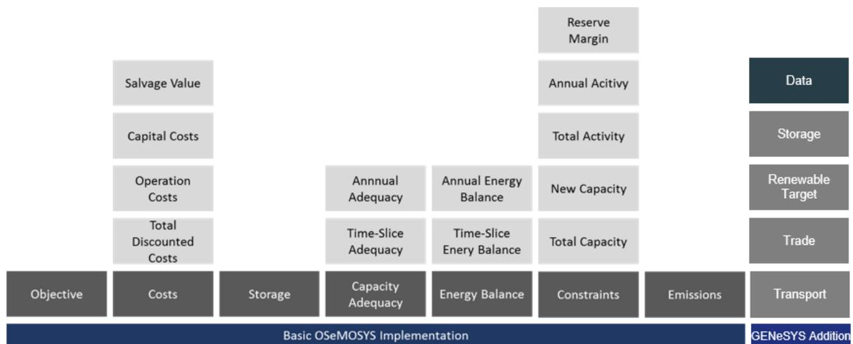
**Figure 1: Blocks of functionality of GENeSYS-MOD**
