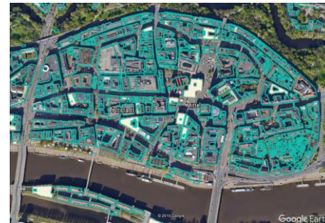
Building models for the State of Bremen rendered in QGIS (via a WMS)
